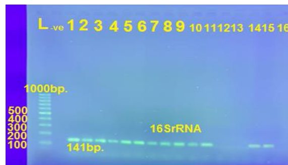
Figure (1): Agarose gel electrophoresis analysis 1% (stained with safe stain) of PCR products presenting partial specific primer (16srRNA) that showed the expected size 141 bp. Lane L: is 100 bp DNA Marker; Lane 2 is (-ve) negative control, Lanes 3-16: samples amplified from h. pylori genome run on 75V for 45min. samples number 1 to10, 14, and 15 were positive for H.pylori infection, while samples number 12, 13 and 16 were negative.
